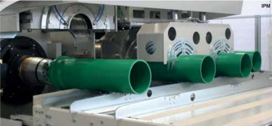
machines (up to 924 sockets per hour for 50-mm diameter x 1.8 mm), end-of-line management (collection, automatic packaging and conveyance to storage of a huge amount of pipes) is increasingly necessary. Moreover, an automated quality control (checking the correct position of the automatically inserted gasket) and socket tightness check system is also displayed, demonstrating that only the pipes that pass inspection are conveyed to the automatic packaging unit.
