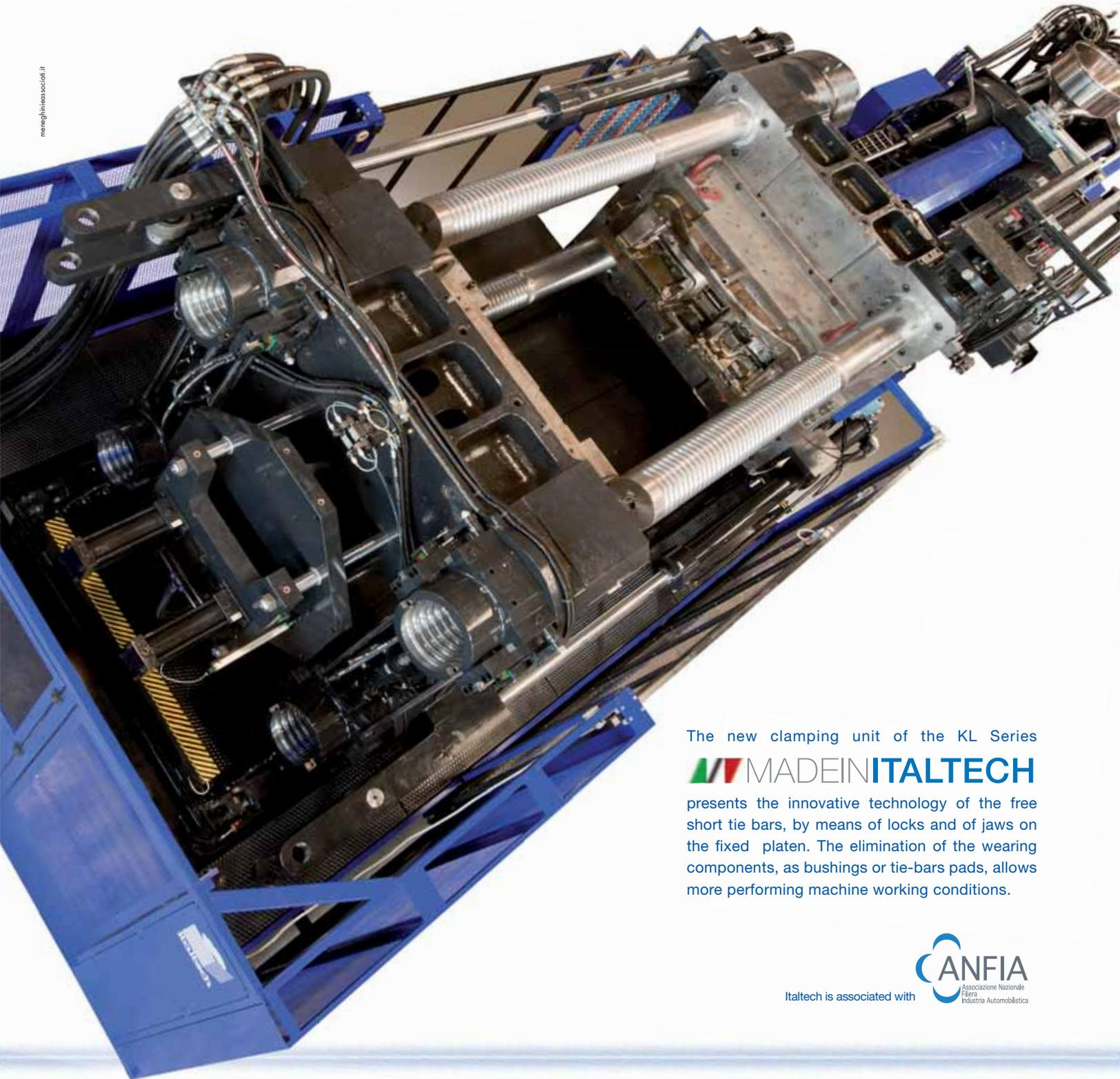
The new clamping unit of the KL Series
